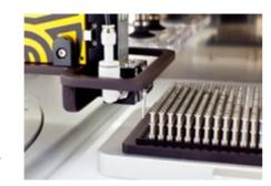
THE SHUTTLE The Shuttle is an accessory to The Stinger that has been designed to rapidly speed up the time between pinning cycles. The Shuttle holds two individual pin cartridges and fits easily into the ROTOR pad rim. When the Shuttle is enabled, The Stinger will take sterile pins from one cartridge and once used, reload them into the second cartridge ready to be autoclaved. Without the Shuttle, pins would need to be manually loaded into the cartridge to be reused after sterilisation.
