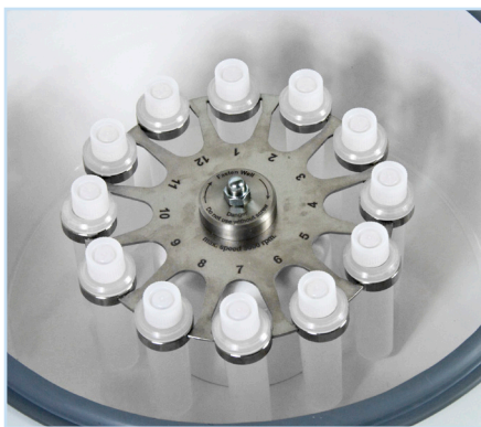
R-12/10, Swing-out rotor for round bottom centrifuge tube
